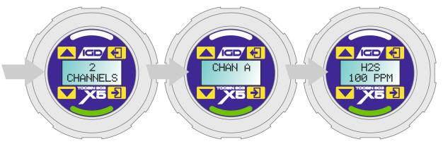
The status indicator stays green if the gas detectors are connected otherwise a channel fault is indicated for the affected channel. The display shows the number of channels and then their type and range
