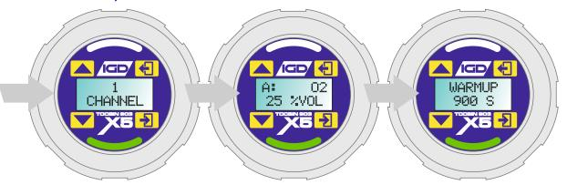
During warm up information is displayed to show the setup of the 903X5. If two channels are fitted information is displayed sequentially.
