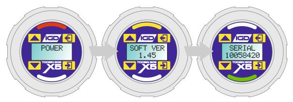
On power up the display back light will show blue with the status indicators cycling red, yellow, green. The display shows the software version and serial number
